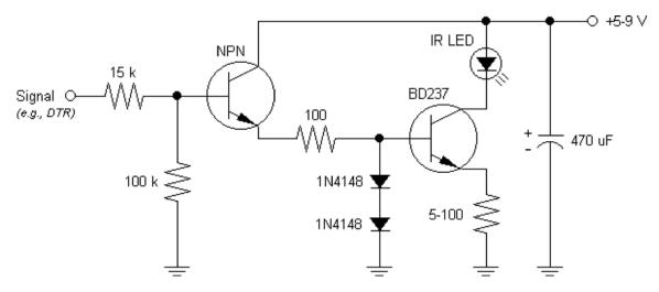
R in the amplifier circuit can be chosen as small as 5 Ohm (for 5V!). Since the signal is pulsed and with a 40kHz carrier frequency, an LED like the LD 271 (or others with max. 100 mA) can tolerate 1A for a short period of time. Some data sheets might mention how high the current can go for certain pulse lenghts.
